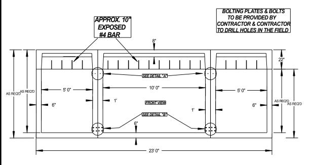
MFG. PER ASTM C478-4000# REINFORCED CONCRETE IN 28 DAYS
